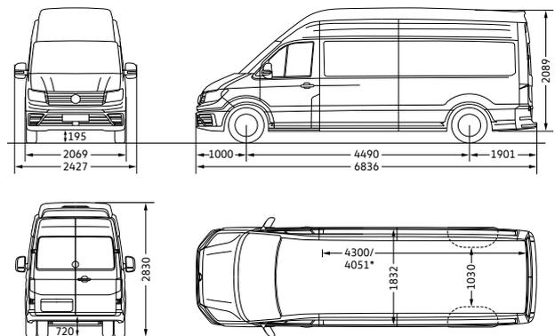
Crafter 50 Delivery Van long wheelbase with overhang and high roof
